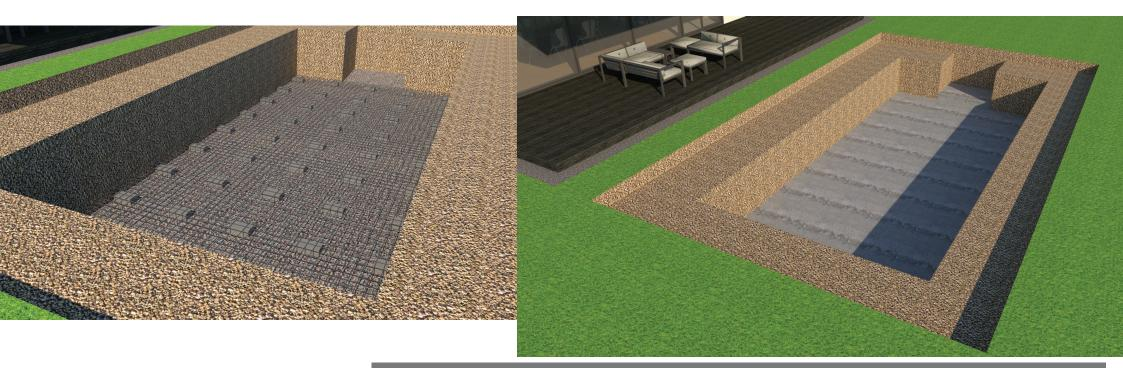
In the case of an overflow pool, it is necessary to maintain the flatness of the base plate +/- 2 mm.
