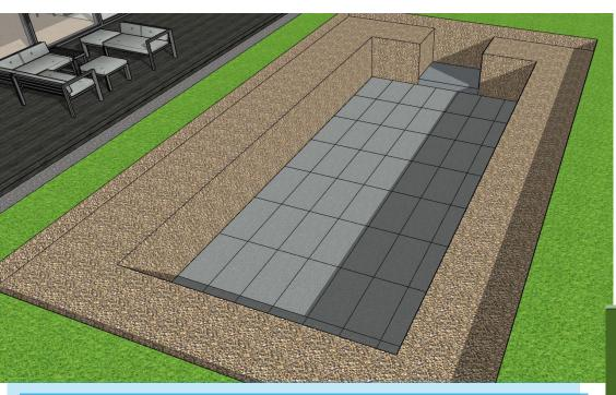
Attach 30 mm XPS extruded polystyrene to the base plate with the help of mounting foam or adhesive tape, polystyrene must always be under the whole swimming pool, including the ribbing.
