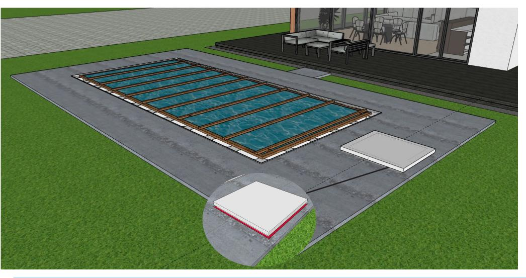
Concreting the top plate around the pool can be done at once, the overflow channel must be concreted min 30 cm. It is necessary to reinforce the concrete slab around the pool with steel net with meshes of 10x10 cm and at least 5 mm thick. The thickness of the top plate should be at least 15 cm in order to be ready for installation of rails for swimming pool enclosure.
